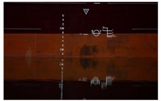
take the readings, and, if safe send photographs from a mobile phone, or could a boat be used to avoid the risks associated with putting a seafarer over the side of the vessel on a ladder? If the only feasible option is to use a ladder to enable draught marks to be viewed, a full risk assessment should be conducted with reference to the vessel's Safety Management System (SMS) before that operation is undertaken.
